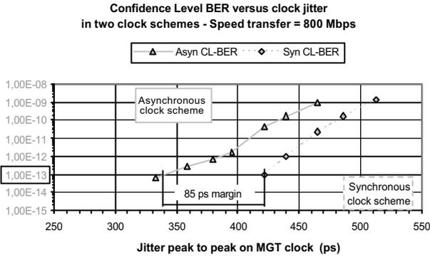
Figure 5 : BER measurements
