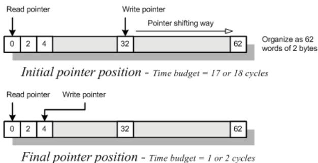
Figure 1 : Elastic buffer pointer positions after the reset and the low latency setting.
