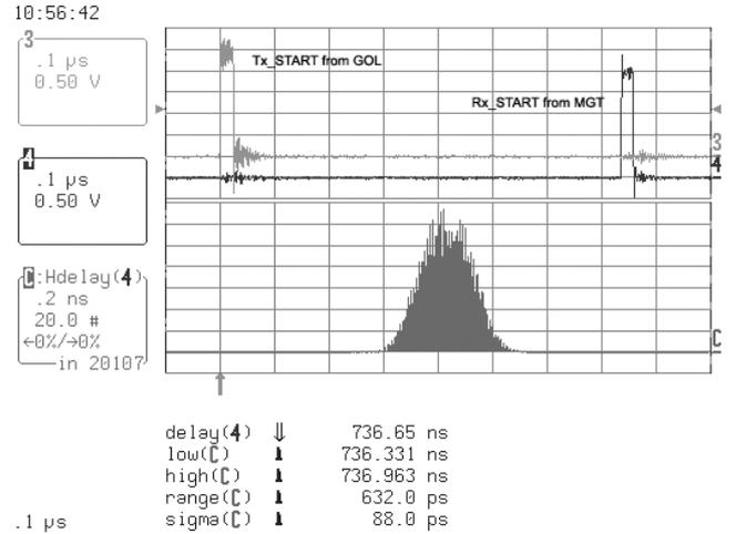
Figure 8 : Latency delay distribution in the synchronous mode. The Gaussian shape, of this jitter, characterizes a pure random source.
