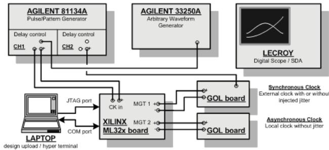
Figure 2 : The test platform
