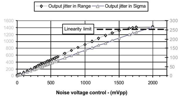
Figure 4 : Transfer function of the pulse/pattern generator. The left/right vertical scales give the jitter range (ps) and the jitter sigma dispersion (ps).
