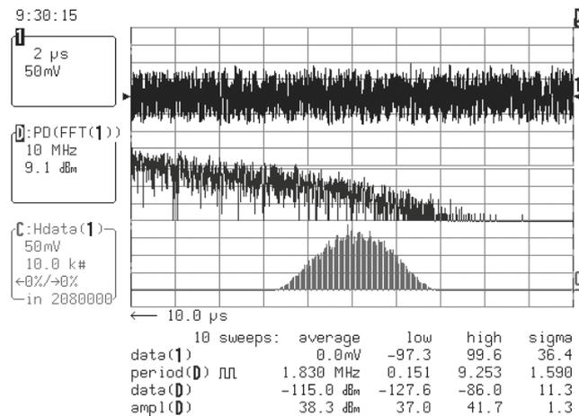
Figure 3 : Injected noise analysis. The upper waveform gives the time domain. The middle one show the frequency domain (Power Distribution with a FFT) and the lower one depicts the Probability Density Function (PDF) of the noise which as expected has a Gaussian shape.
